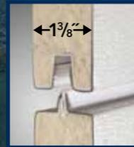
A Full Thermal Break is used in the tongue-and-groove construction of all 600 series doors. This rigid vinyl extrusion seals the joints and eliminates metal-to-metal contact, which limits the transfer of temperature.
